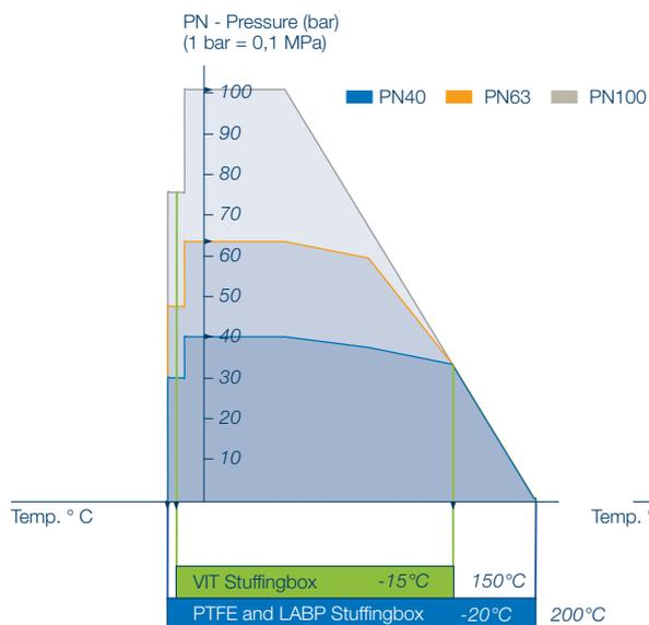
PT diagram for the sealing elements SS
