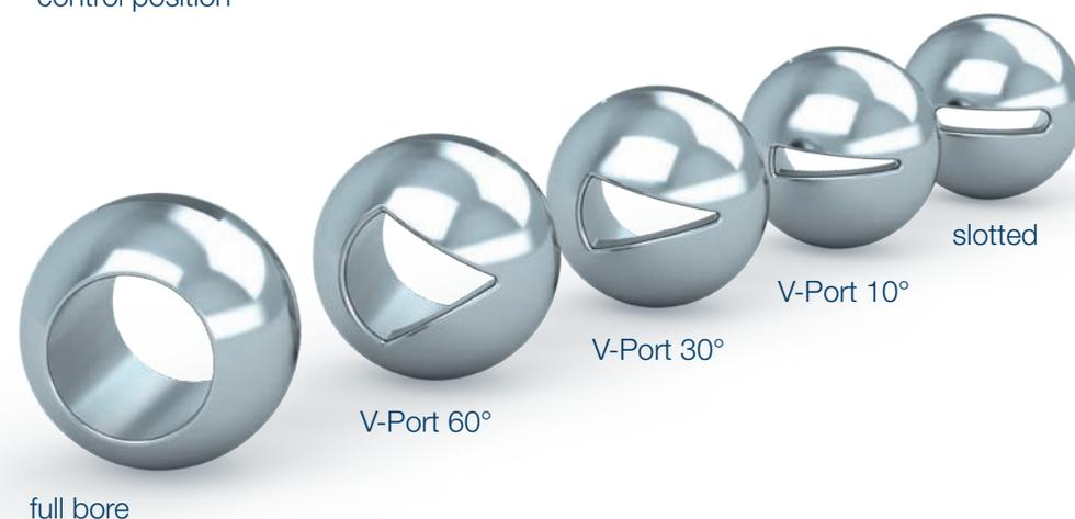
This V-cut gives this V-port ball valve its name. The size of the V-port regulates the flow rate – from full bore to sectioned 10°, 30° and 60° as well as slotted
