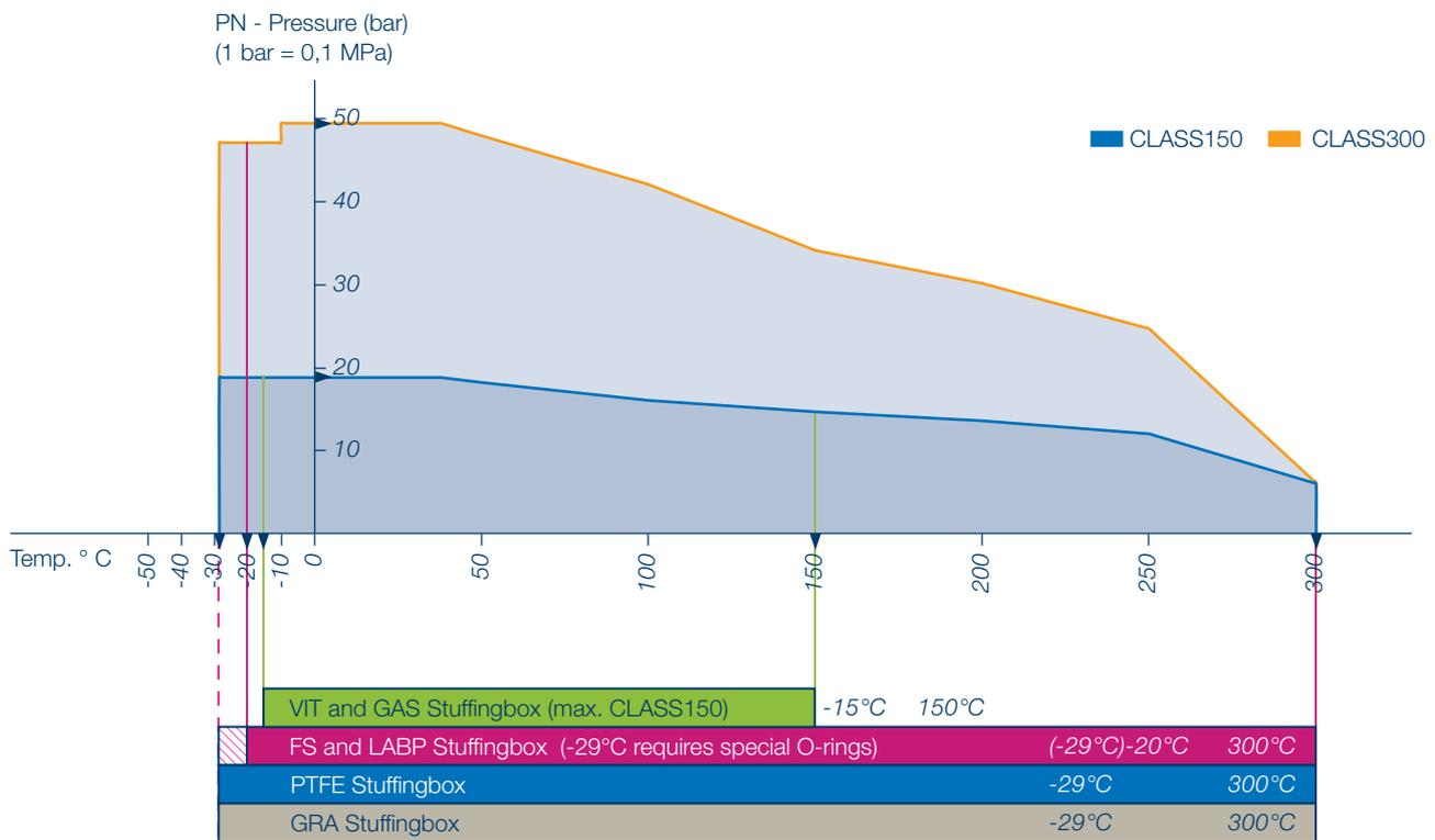
PT diagram for the sealing elements PP
