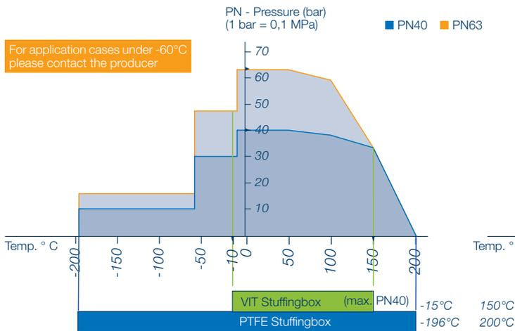
PT diagram for the sealing elements SS
