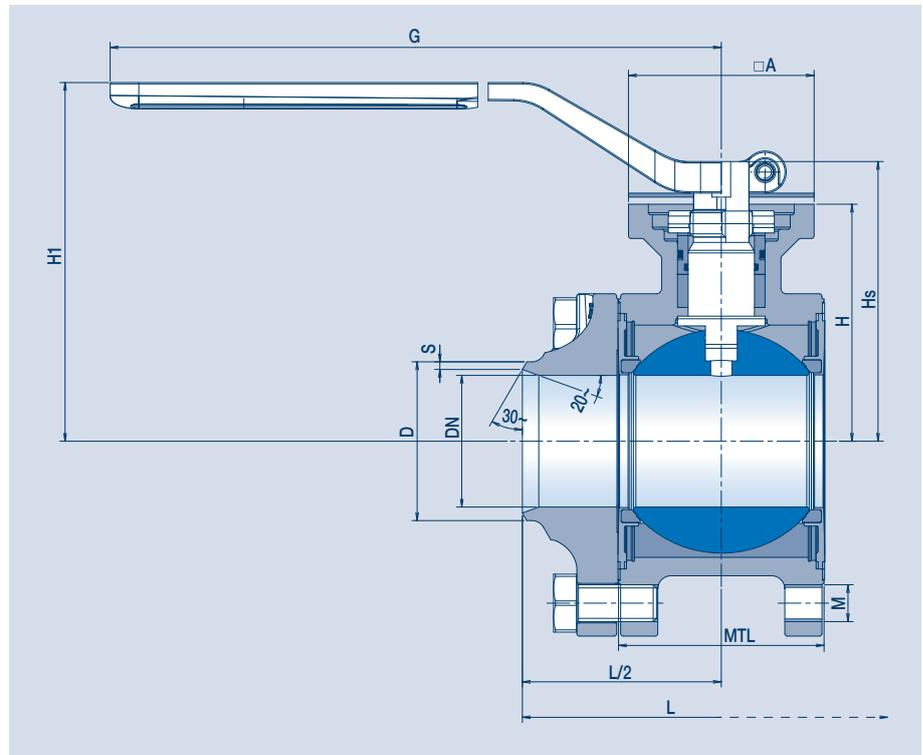
**NOTICE: DOES NOT HAVE TO BE DISMANTLED WHEN WELDING INTO THE PIPELINE**
