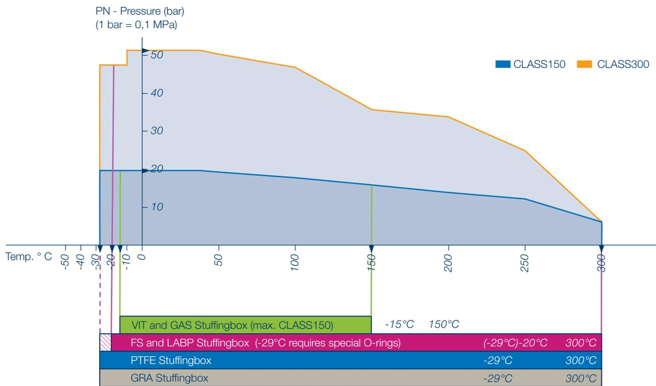
PT diagram for the sealing elements PP
