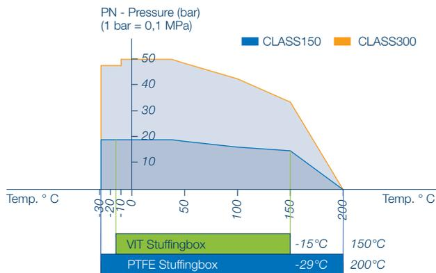
PT diagram for the sealing elements SS
