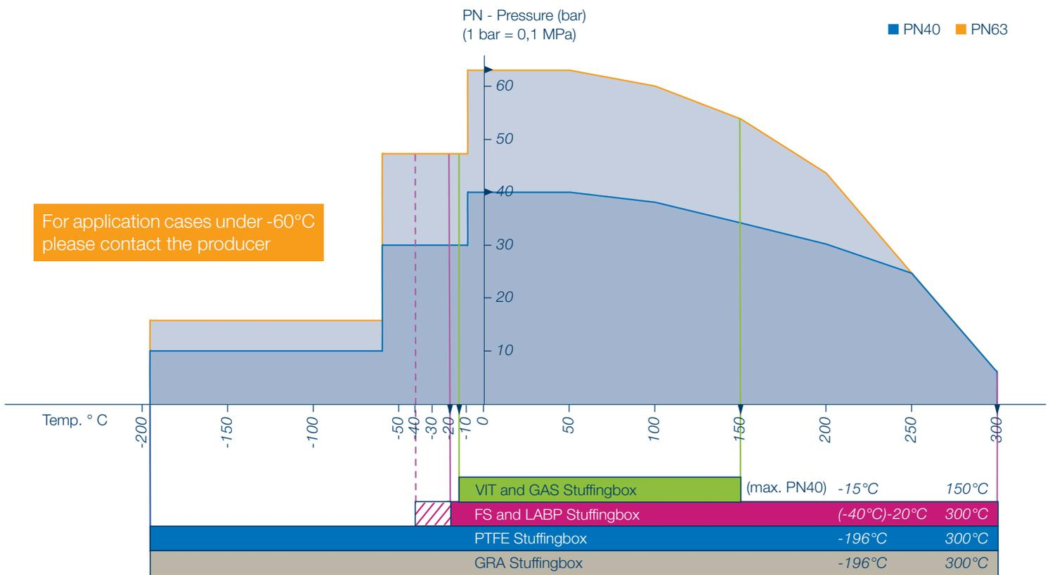
PT diagram for the sealing elements PP
