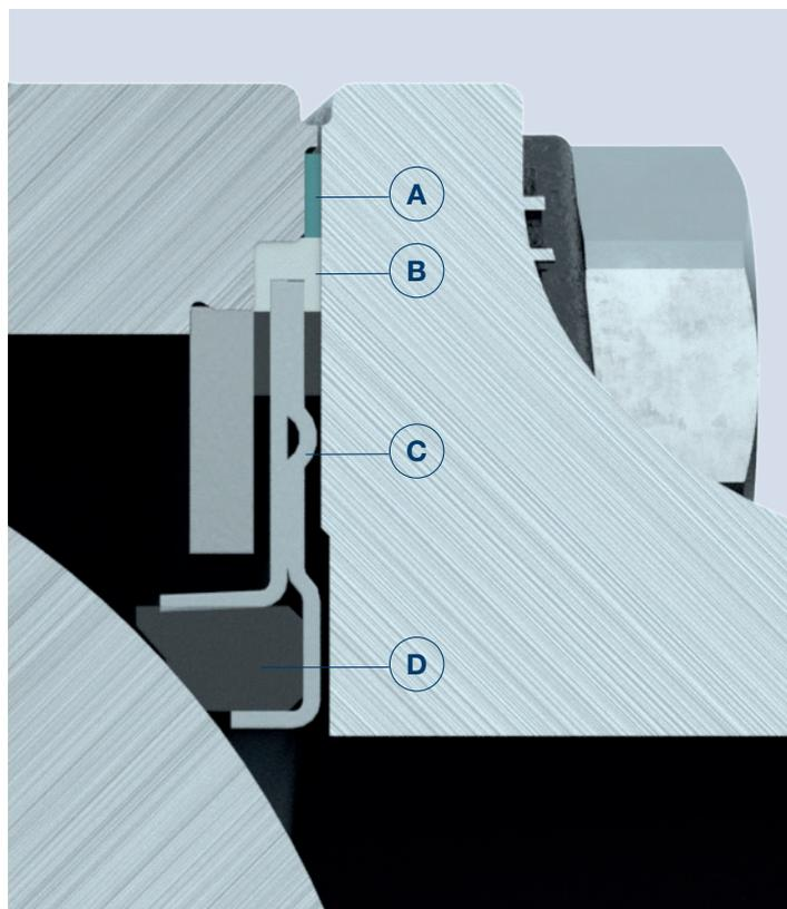
accordance with the KLINGER standard! The fiber-reinforced sealing ring KLINGER KFC-25 consists of PTFE and graphite and is surrounded on three sides by the spring-loaded sealing element. It can thus absorb large amounts of contact force without deformation and is simultaneously protected against the medium.
