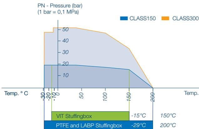
PT diagram for the sealing elements SS
