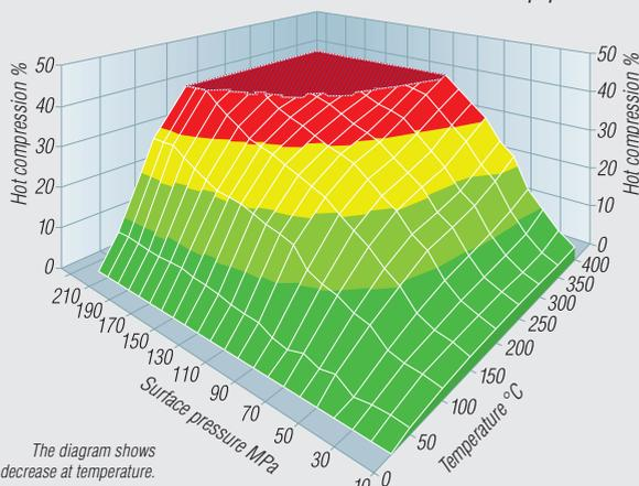
The diagram shows additional thickness decrease at temperature.
