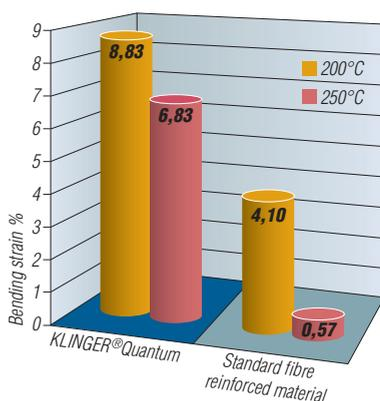
The unique behaviour of KLINGER® Quantum manifests itself even more impressively in long-term tests. For this purpose, a fibre-reinforced reference material, together with KLINGER® Quantum was again treated at a temperature of 200°C for 300 h and 600 h.
