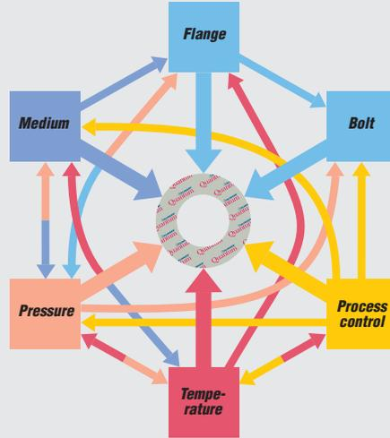
Maximum temperature and pressure values alone can not define a material's suitability for an application. These limits are dependent upon a multiplicity of factors as shown in the diagram opposite.
