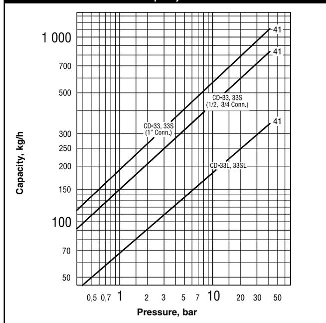
**Note:** CD traps can operate with minimum of 0,15 bar inlet pressure and a maximum of 80% back pressure. However, for best results, inlet pressure should not drop below 0,70 bar and back pressure should not exceed 50% of inlet pressure.
