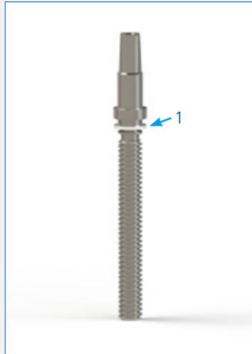
**04:** Stem and collar made in one piece in stainless steel for **better resistance to axial load and to withstand higher operating torques**. A polyamid washer (1) placed under the collar allows to reduce friction torque and protect coating inside the Bonnet.
