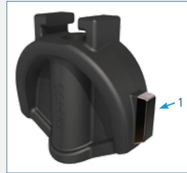
**07: Male guiding system with composite sliding skate (1)** reduces the wear of the wedge against the body, allowing a smooth functionality and a longer life time of the valve. Furthermore, the increased thickness of the elastomer at the sealing areas improves product resilience to the usual small impurities encountered in networks.
