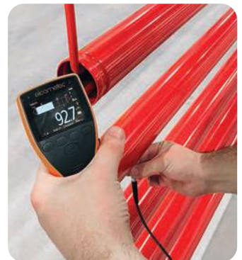
Layer thickness control
