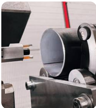
Automatic pipe seam detection & positioning
