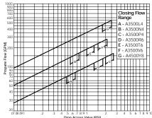
NOTE: Multiply flow rate by .94 to determine liquid butane flow and by .90 to determine liquid anhydrous ammonia flow
