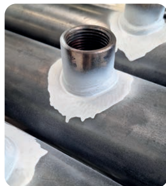
Liquid penetrant testing
