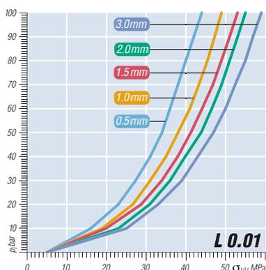
Tightness class  $L = 0.1$  allows a maximum leakage of 0.1 mg nitrogen per second per meter of gasket length (mg/s x m)
