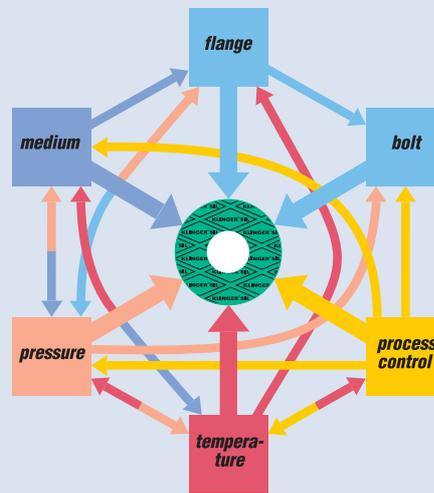
Maximum temperature and pressure values alone can not define a material's suitability for an application. These limits are dependent upon a multiplicity of factors as shown in the diagram opposite. It is always advisable to consider these factors when selecting a material for a given application.
