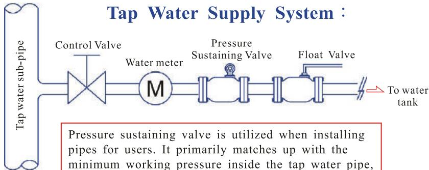
Pressure sustaining valve is utilized when installing pipes for users. It primarily matches up with the minimum working pressure inside the tap water pipe, balancing up-stream and down-stream pressure during normalcy and emergency, and maintains constant pressure inside the pipe.
