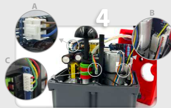
Remove the cables (from the cover) connected to the actuator PCB (Fig. A, B and C).
