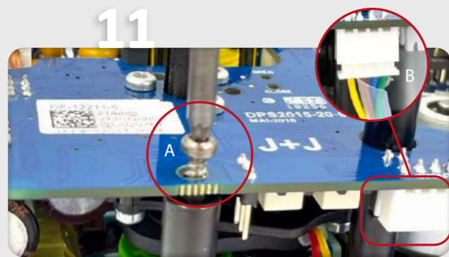
Fix the DPS positioner PCB (Element C) to the plastic column (Element B) with the plastic fixing screw (Element E) (Fig. A). Connect the remaining cable (Element A) to the connector base on the DPS PCB (Element C) (Fig. B).
