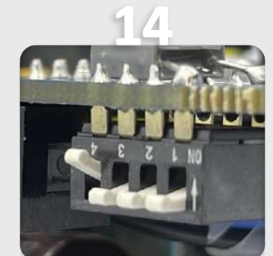
Use the configuration you need by moving the DIPs, according to the instrumentation signal:
