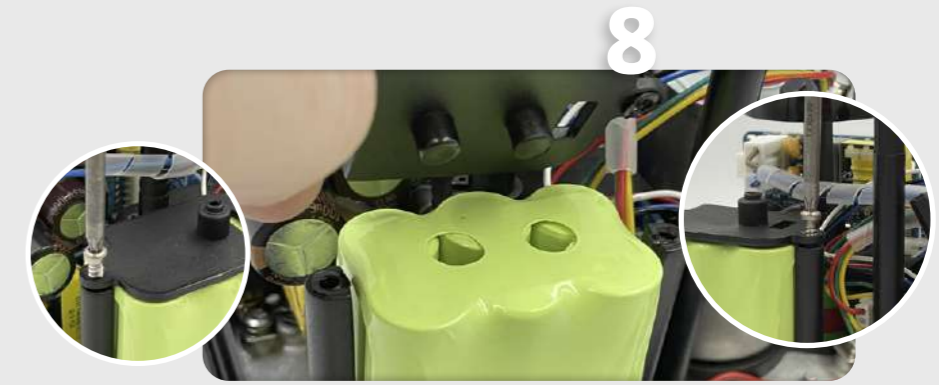
Place the upper battery support and fix it to the columns of the lower battery support (Element B), by using the Plastic fixing screws (Element F).
