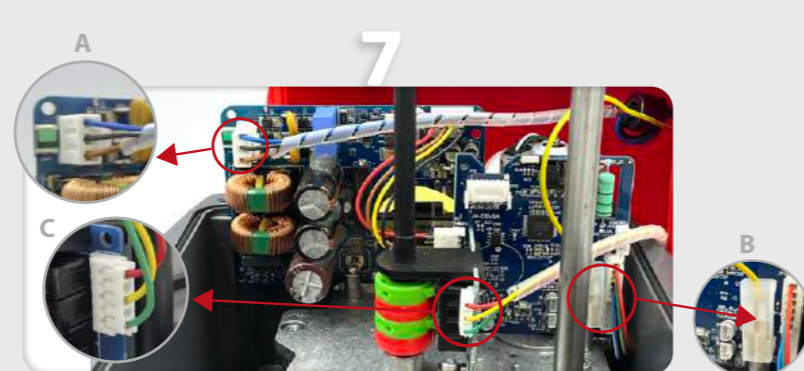
7 Take the DPS cover (Element A) and connect its cables, following (Fig. A, B and C).
