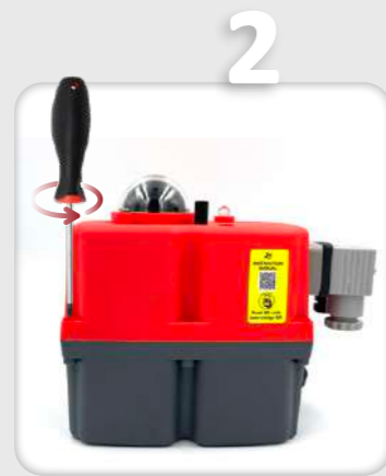
Remove the 6 screws between the cover and the body of the actuator.
