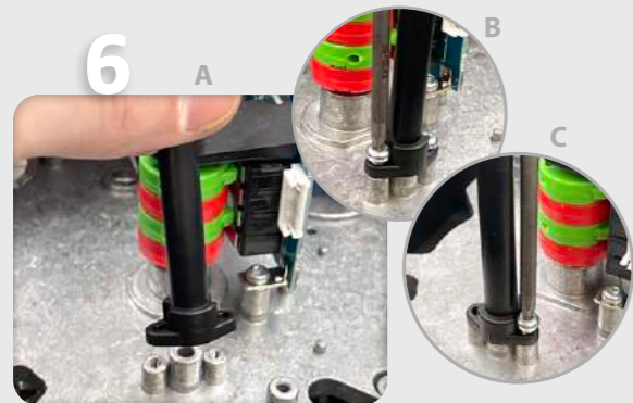
6 Fix the plastic column (Element B) on the base plate, by using 2 sheet metal fixing screws (Element D) (Fig. A, B and C).
