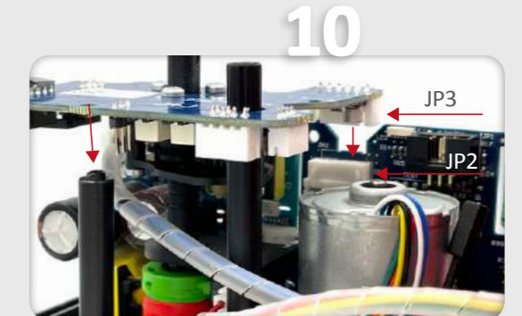
Press the DPS positioner PCB (Element C) along the shaft until the PCB connector (JP3) is plugged in the actuator PCB connector (JP2).
