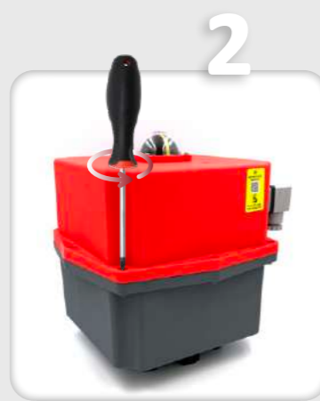
Remove the 8 screws between the cover and the body of the actuator.
