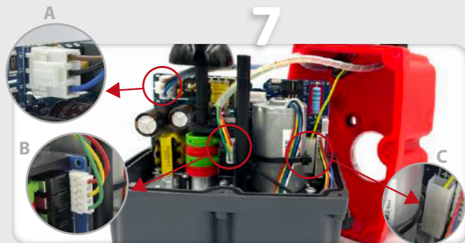
Take the DPS cover (Element A) and connect its cables, following (Fig. A, B, C).
