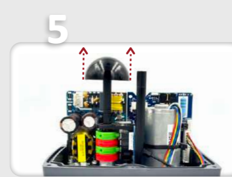
Carefully remove the position indicator.
