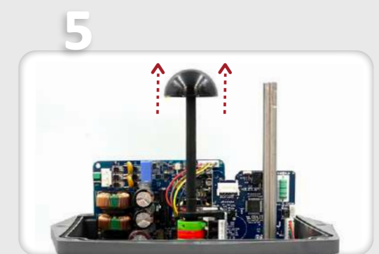
5 Carefully remove the position indicator.
