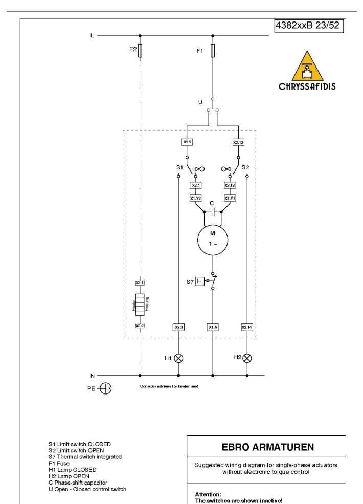
The valve is in intermediate position!
