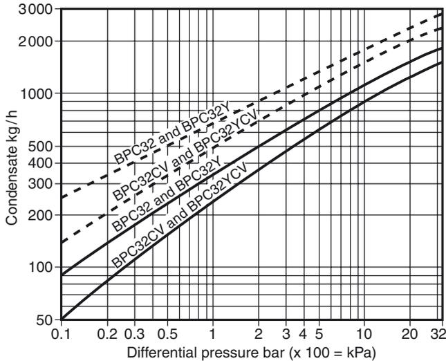
Hot water capacity ——— Cold water capacity - - - - -
